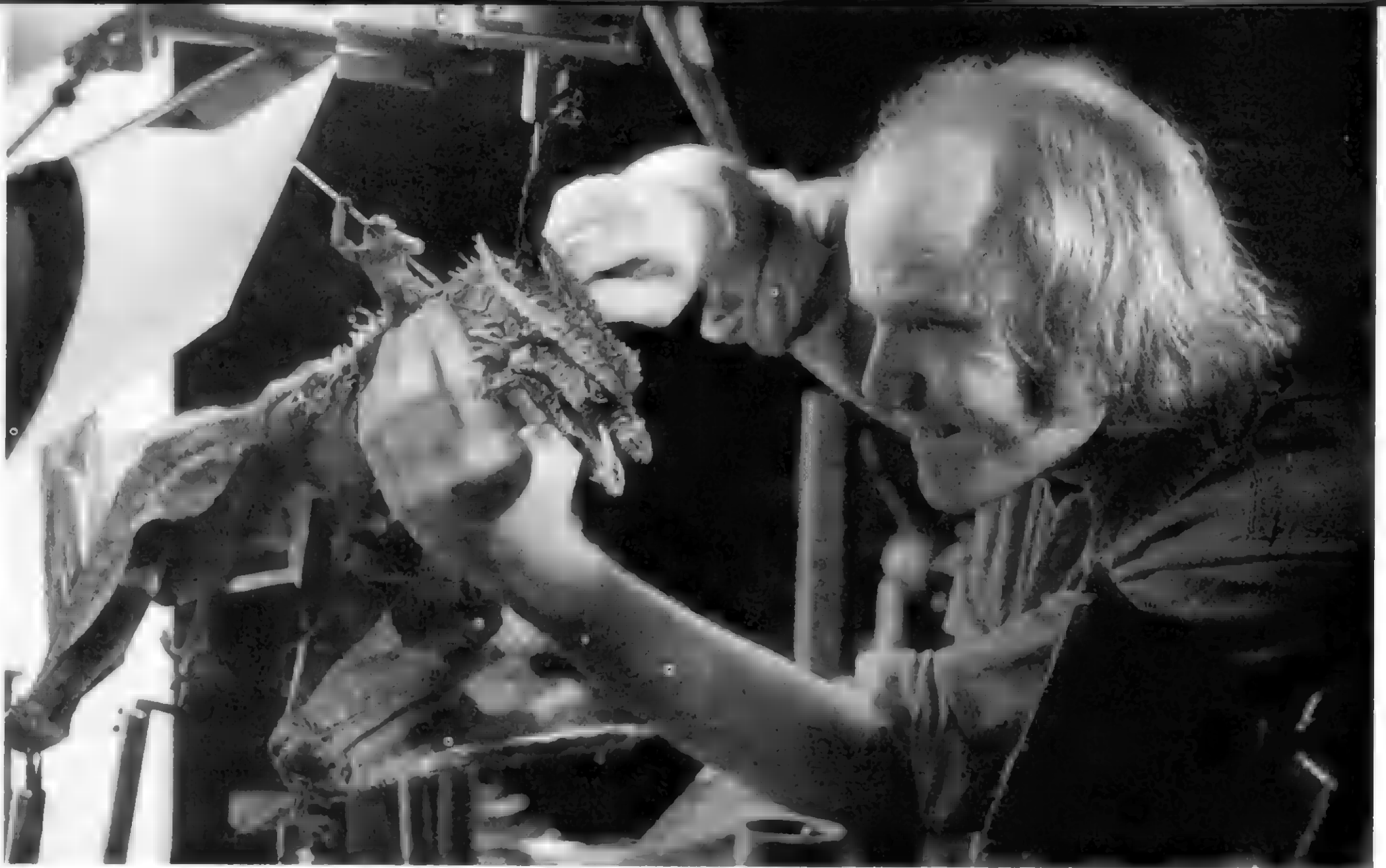
Phil Tippett works with the go-motion dragon at Industrial Light and Magic during the filming of Dragonlayer . The feet and head of the dragon are connected to motorized rods, but some small movements of the mouth and the figure are made with traditional stop-motion.
